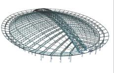
The arena roof is part of the King Saud University Sport Campus in Riyadh (Saudi Arabia) and it is the main feature of the sport campus. The building is for indoor athletics and also has the ability to hold conferences. The basic form of this building consists of a large single span roof with a central arch truss supporting secondary trusses.
