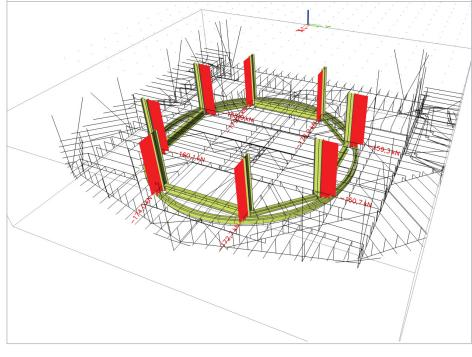
The revolving stage in the new Music Theatre Linz is a two-storey steel construction with an outer diameter of 32 m. The height of the two storeys is 3.95 m and is adapted to the surrounding building. The space underneath the revolving stage is used as an underground parking garage.
